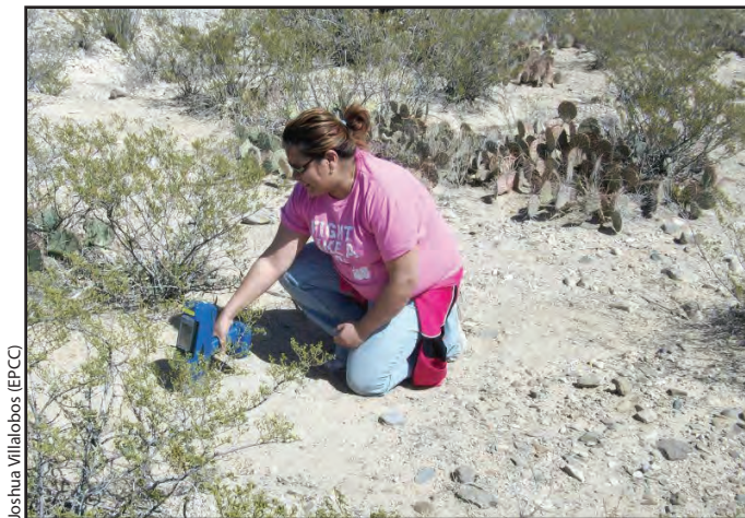
Marie Gomez (EPCC) using a Portable X-ray fluorescence (XRF) to locate pollutants in desert sediments around El Paso, Texas.
