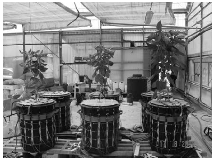
Picture of experimental setup including growth chambers equipped with 96 electrodes each
