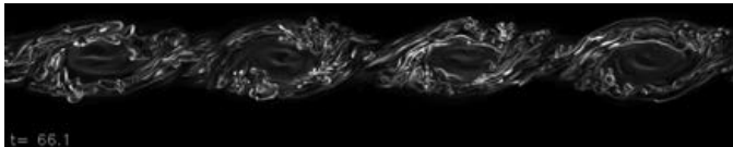
Computed vorticity of turbulence produced by a strong wind shear in the mesosphere.
