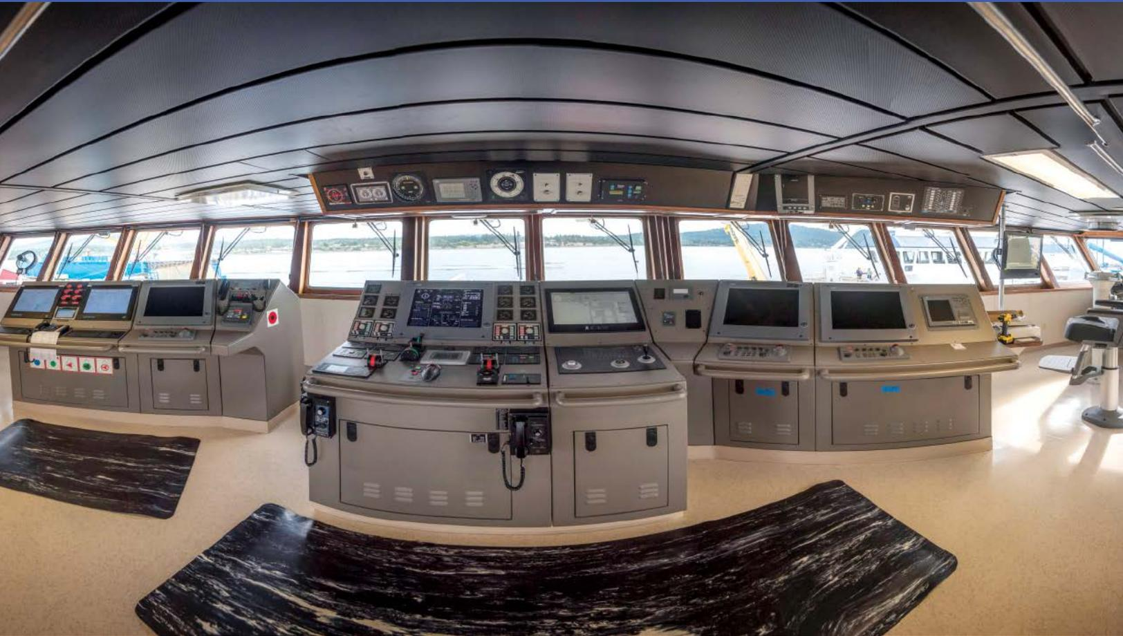
The Pilot House, also called the bridge or wheelhouse is where the ship's deck officers – first, second and third mate, plus the vessel's master – command the vessel.
