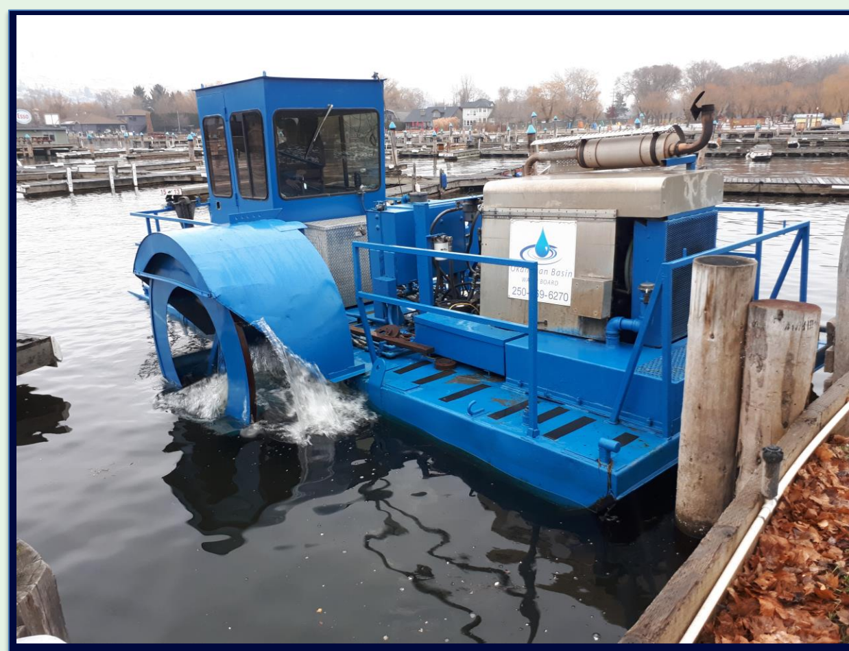
Figure 2. Aquatic rototiller utilized by Okanagan Basin Water Board; used in removing Eurasian watermilfoil roots from Wood Lake, BC.
