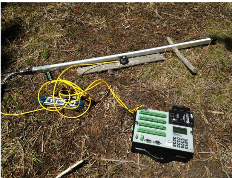
Figure 4. Transect system with a point sensor (PSQ1, Kipp & Zonen, Delft, Netherlands), line quantum sensor (LI-191SL, LI-COR Inc, Lincoln, NE) and a data logger (CR3000, Campbell Scientific, Logan, UT)
