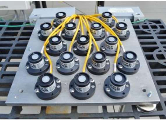
Figure 8. PSQ1 sensors compared to standardized sensor
