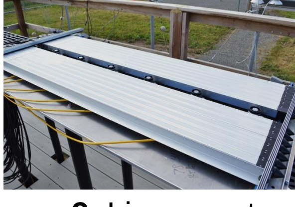
Figure 9. Line quantum sensors calibrated using six standardized point sensors
