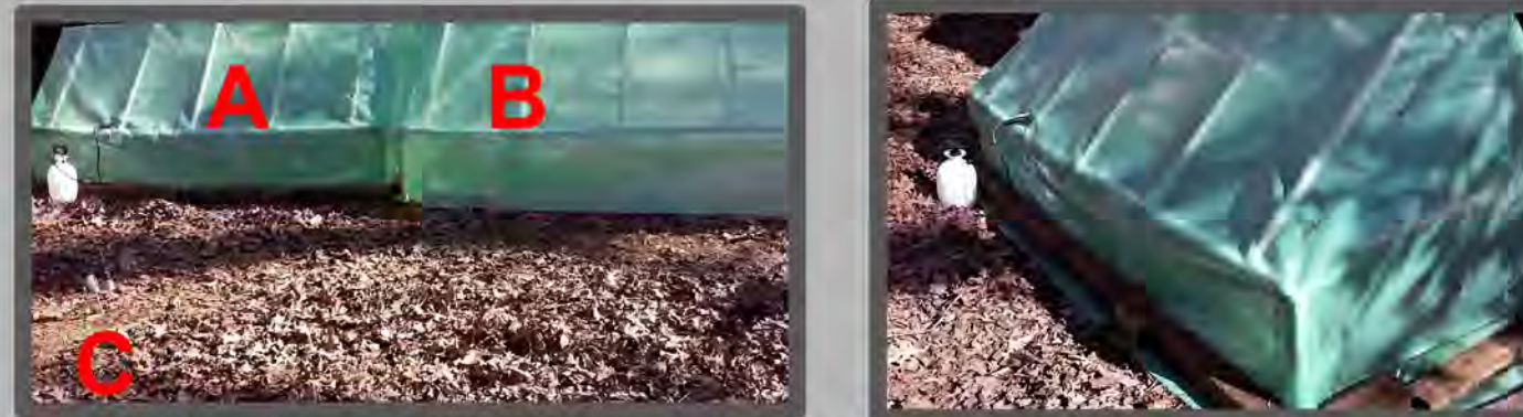
Fig. 2 Sample area A (CO 2 added), area B (enclosed, but no added CO 2 ), and control
