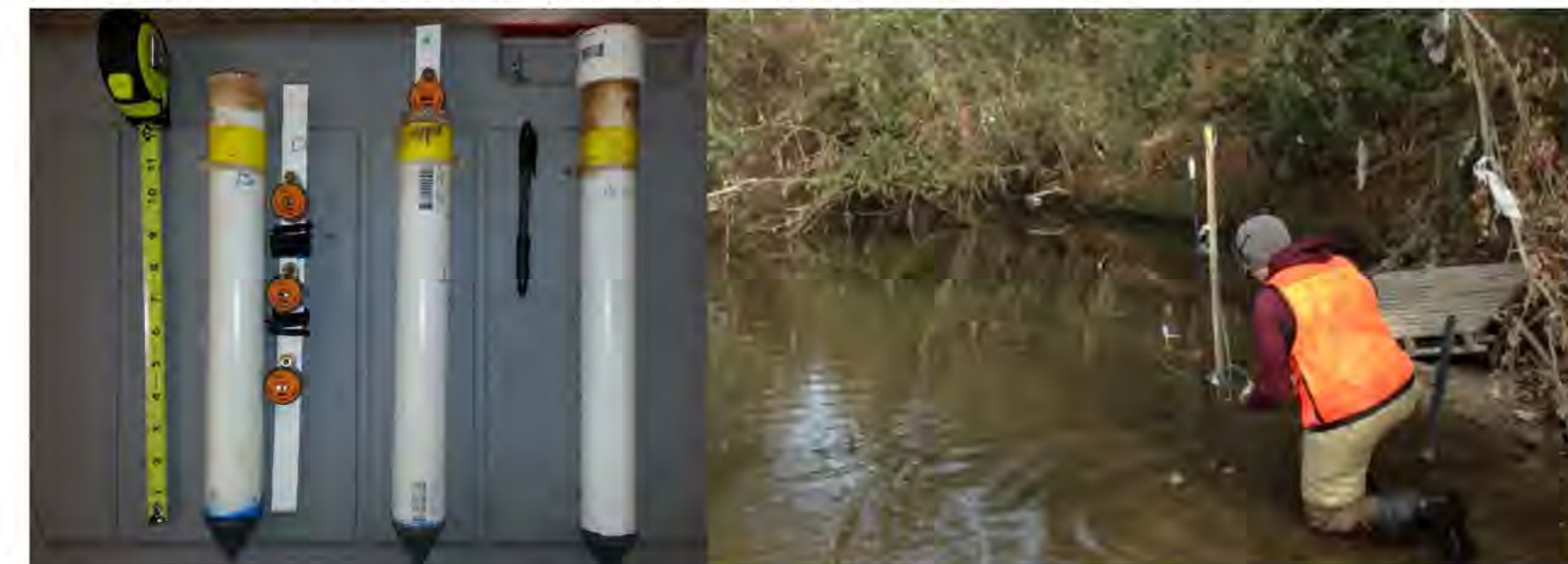
Fig. 2: Thermal profilers were used to collect temperature data (left) while groundwater samples were collected using a piezomanometer (right).
