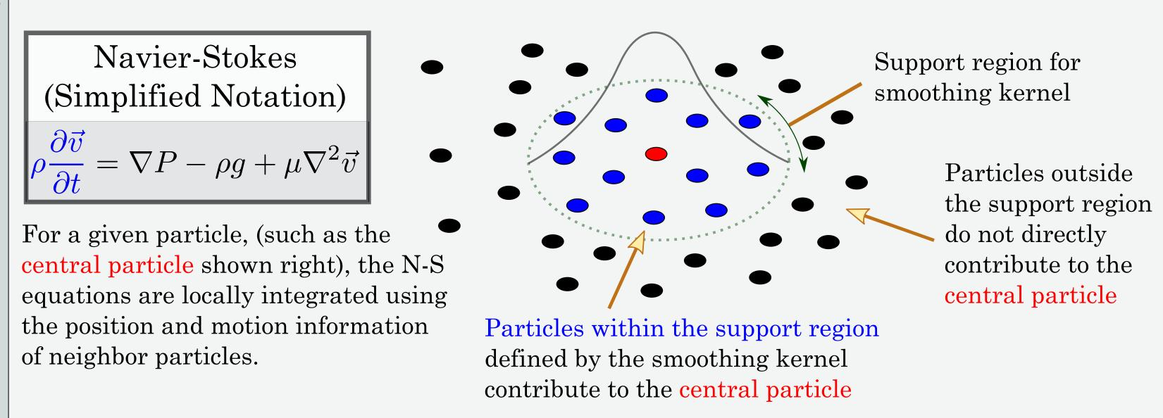
SPH is able to handle the fluid accelerations very well, which allows for realistic simulation of natural flows and fluid-structure interaction.
