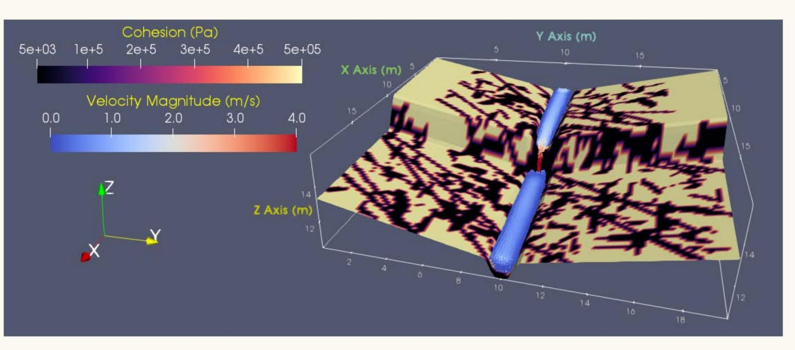
In the above synthetic bedrock channel (20 m \* 20 m with a 2 m vertical drop at the knickpoint), water flows over bedrock with strength heterogeneities which are defined in space by a power law fracture distribution. The small waterfall marks a transition in hydraulic stresses from shear-dominant to normal-dominant.
