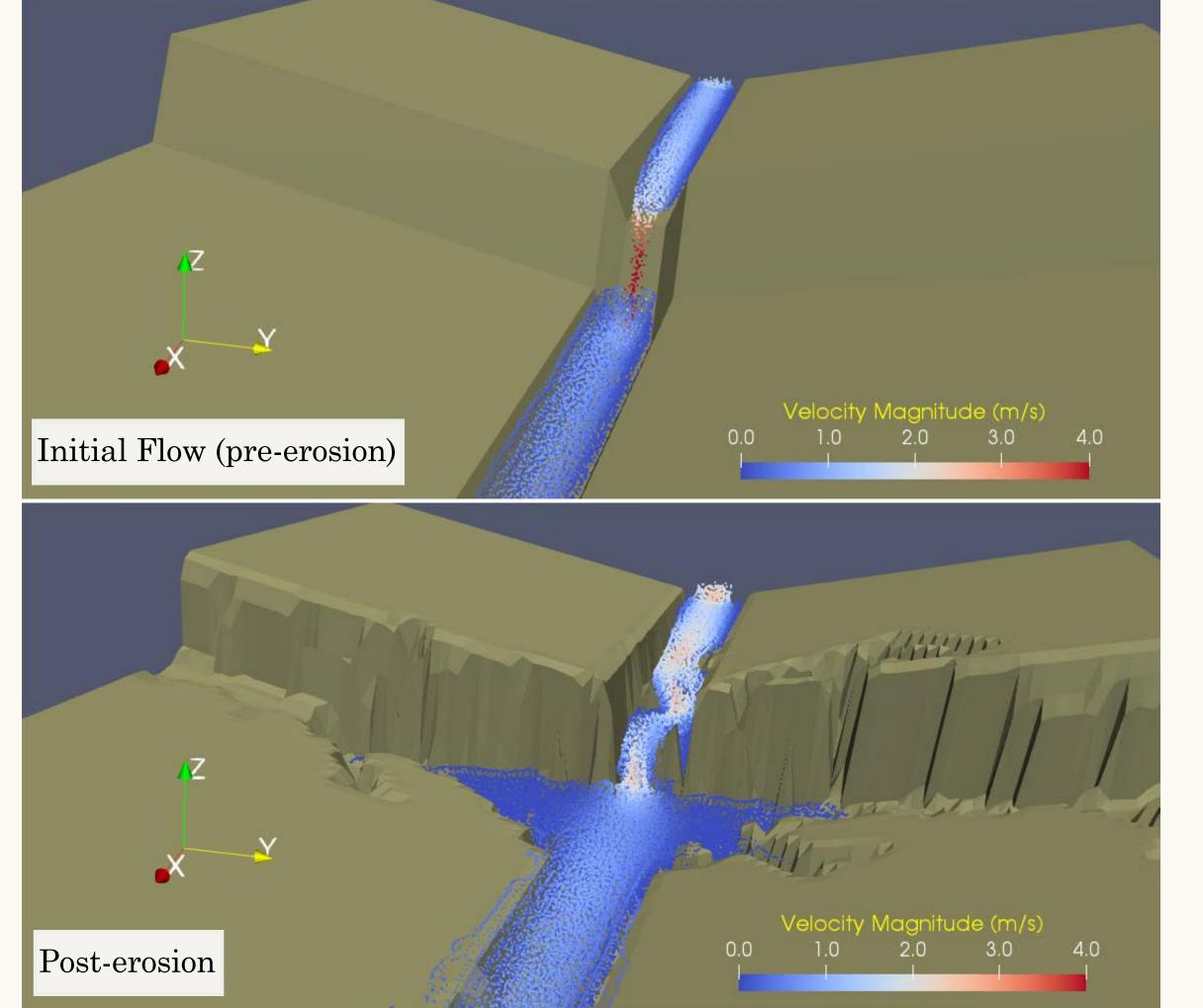
Erosion via coupled FERM-DualSPHysics modeling shows a reorganization of the channel's velocity structure as weak material is preferentially removed from the domain.
