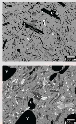
Example back-scattered electron (BSE) images of crystals from early fissure 8 (top) and fissure 17 (bottom). Phases are labeled as V=vesicle, C=crystal, G=glass
