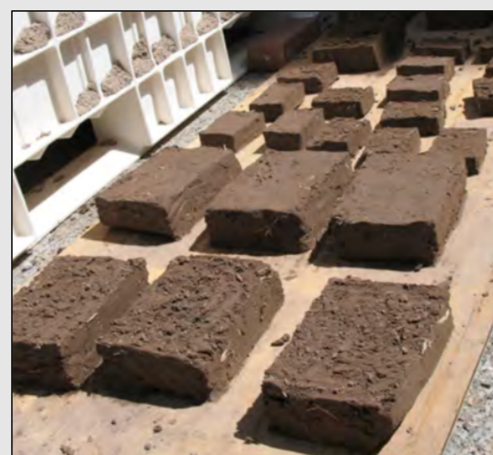
Figure 1. Sisal fiber-reinforced adobe bricks prior to drying at NMSU.
