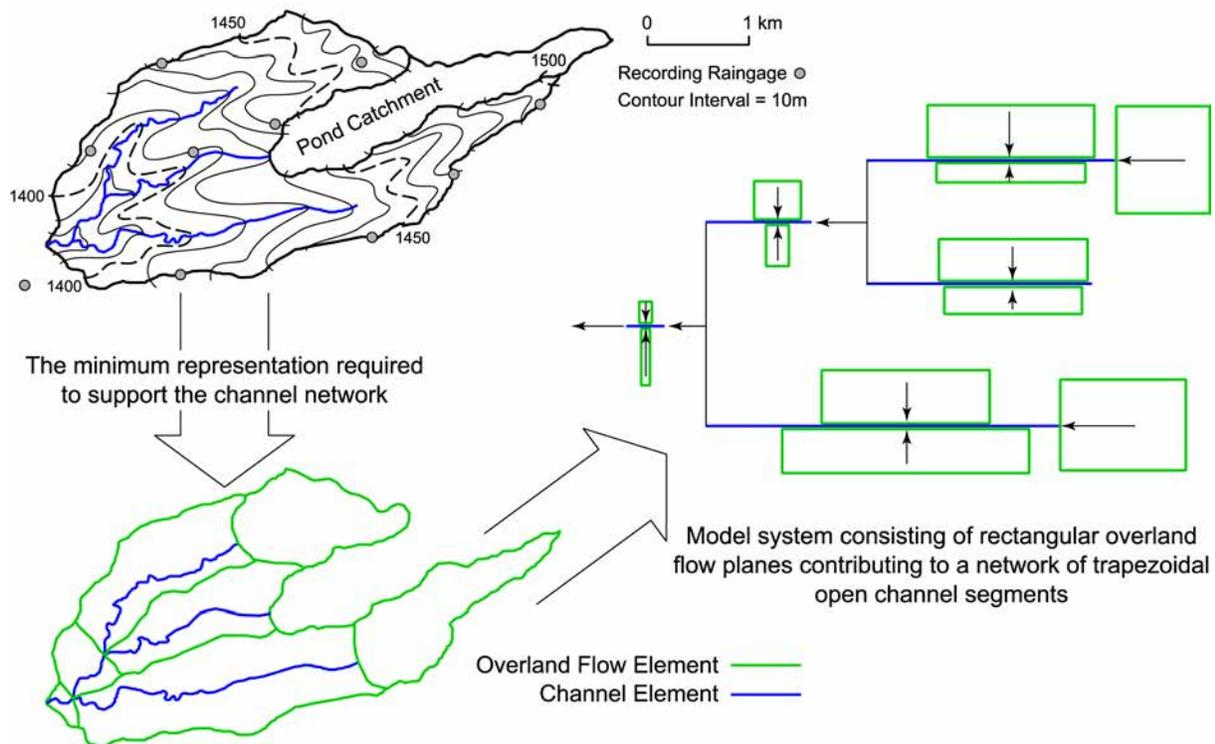
Figure 1. Illustration of how topographic data and channel network topology is abstracted into the simplified geometry defined by KINEROS2 model elements. Note that overland-flow elements (with either curvilinear or uniform slope profiles) are dimensioned to preserve average flow length, and therefore the width of overland flow elements contributing laterally to channels generally do not match the channel length.
