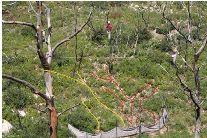
Figure 1: Erosion plot (silt fence) on the equatorial-facing slope; connected rills and flow patterns are marked.
