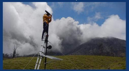
Dr. Maarten de Moor performing maintenance on one of the NOVAC DOAS scanners installed at Turrialba that OVSICORI uses to monitor  $SO_2$  emissions in real time.
